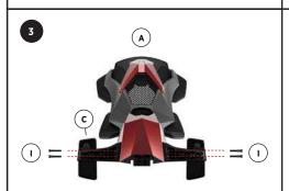
Attach Armrests: Attach them to the seat frame using screws (provided). Make sure they are securely fastened.
