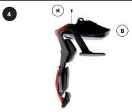
Attach Backrest to Seat: Place the seat upside down on a flat surface. Align the mounting holes. Use screws to attach the backrest to the seat. Again, tighten the screws evenly for stability.
