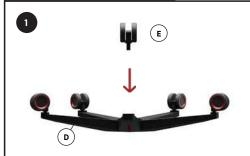
Attach Casters to Base: Simply insert the stem of each caster into the holes in the base and push until they snap into place. Make sure they are securely attached.
