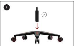
**Attach Gas Lift Cylinder:** The gas lift cylinder is responsible for adjusting the height of the chair. Slide the gas lift cylinder into the center hole of the chair base. It should fit snugly.
